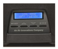
Local User Interface: Can be used with Main Control for adjusting settings, reading temp/humidity, and reading fault codes at the unit.
