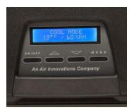
The control has been wired and set up in the factory for testing with default settings. It is an electronic digital thermostat for one-stage cooling. No additional adjustments should be necessary except adjusting the cellar temperature to your preference. If additional adjustments or changes are necessary, please refer to the configuration settings section in this manual.
